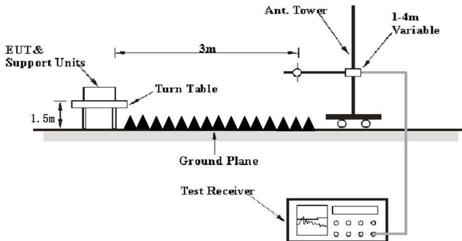
The radiated emission tests were performed in the 3 meters test site, using the setup accordance with the ANSI C63.10-2013. The specification used was the FCC 15.209, and FCC 15.247 limits.
