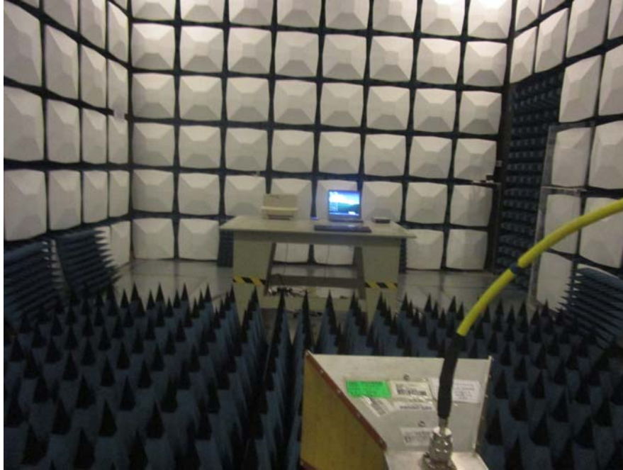
Radiated Emission Front View (Above 1GHz)
