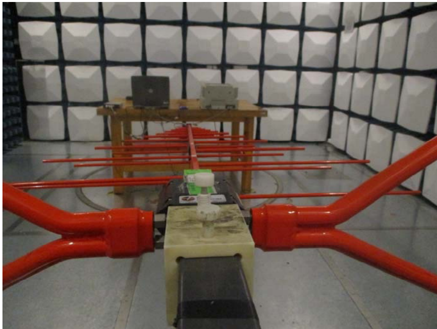
Radiated Emission Rear View (Below 1GHz)
