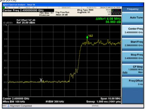
Test Plots with hopping ( $\pi/4DQPSK$ )
