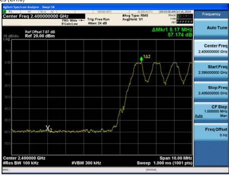
Test Plots with hopping (GFSK)
