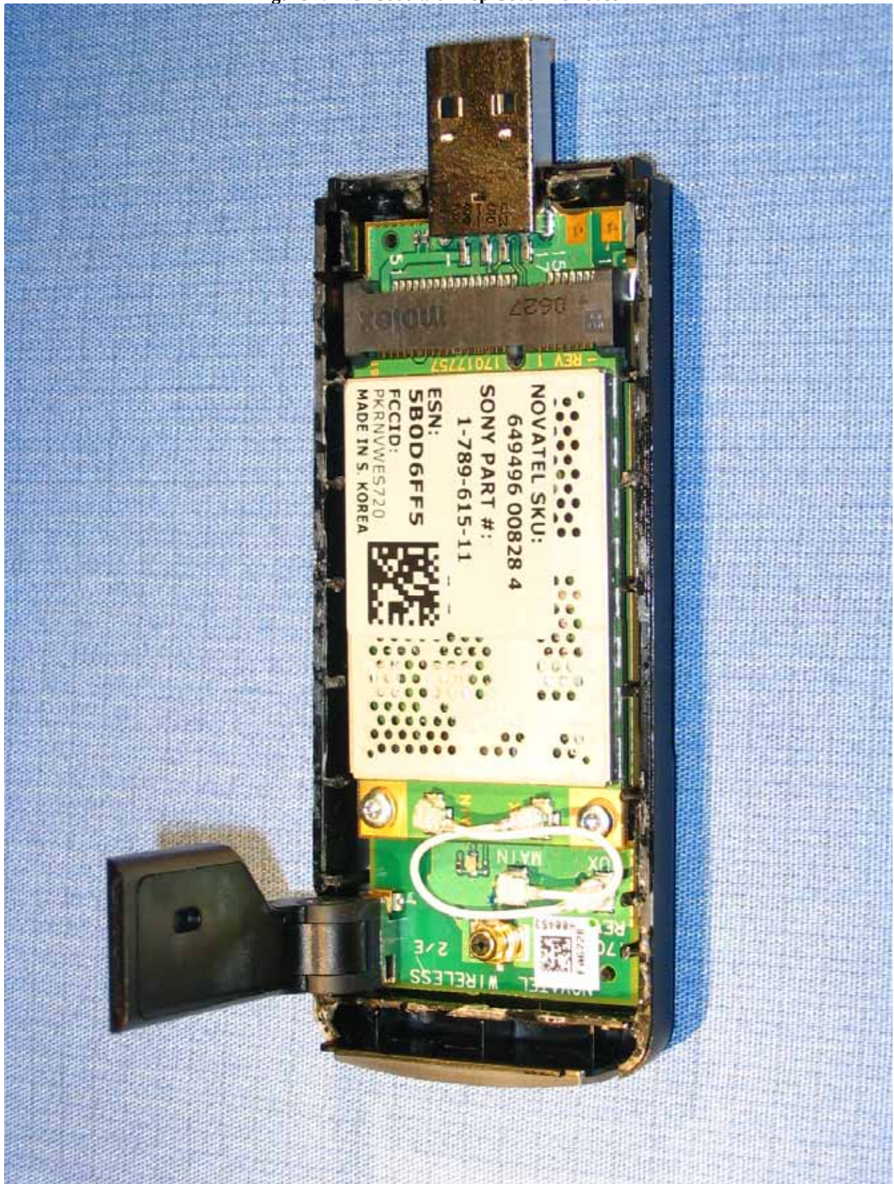
Figure 1: MCD3000 with Top Cover Removed
