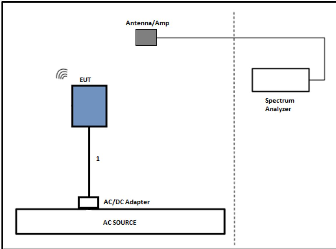
**TEST SETUP- AC LINE CONDUCTED:**
