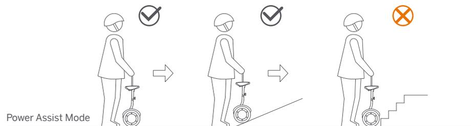
Pull up the guide bar to enter Power Assist Mode (powered on, with no rider).
