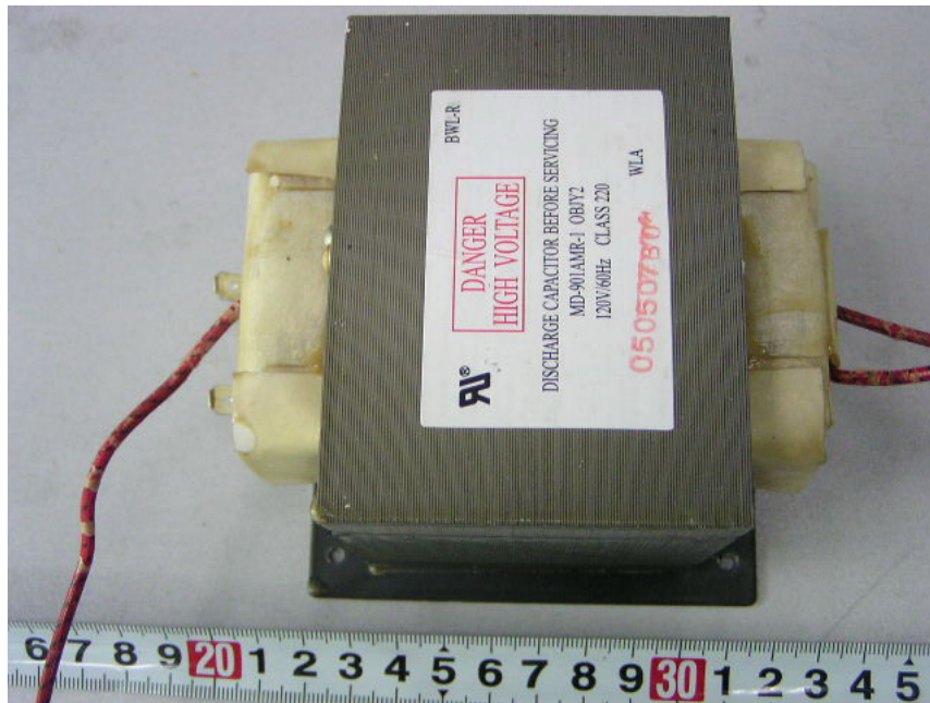
EUT- Transformer View
