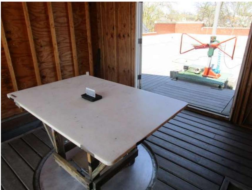
RADIATED EMISSIONS TEST SETUP 1 TO 18 GHZ
