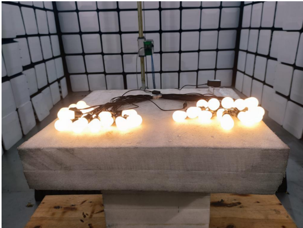
Photo of Radiation Emission Test
