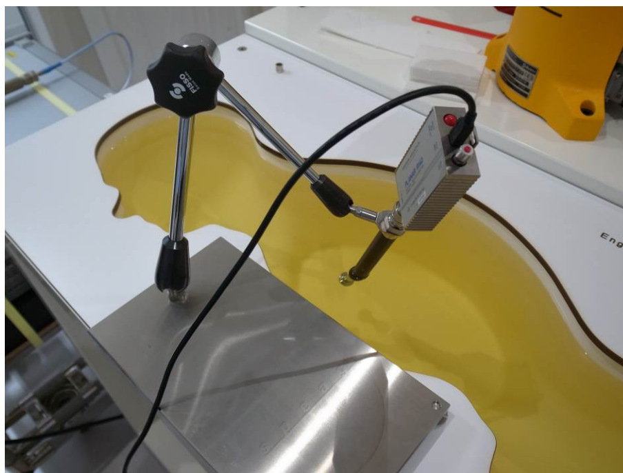
(b) Example Photo: Dielectric Parameter Measurement
