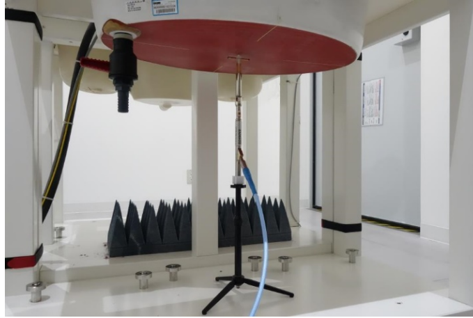
(c) Photo: System Validation Dipole Placement
