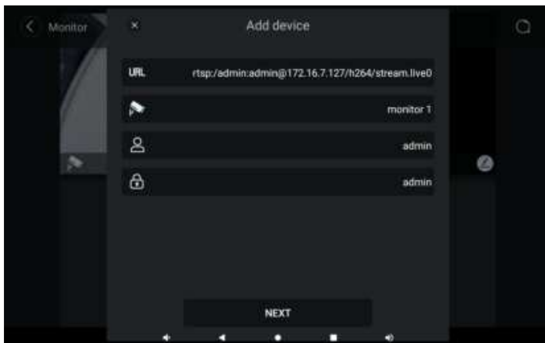
Picture 23 - Configure device monitoring
