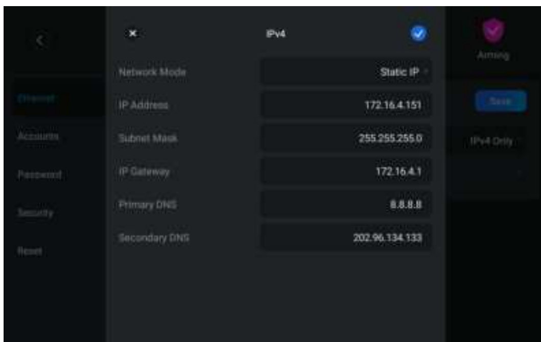
Picture 82 - Static IP network mode
