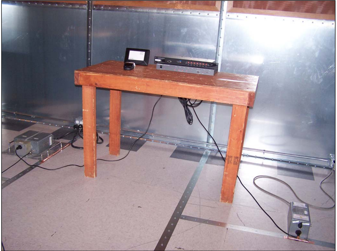
Photograph 1. Conducted Emissions Limits, Test Setup
