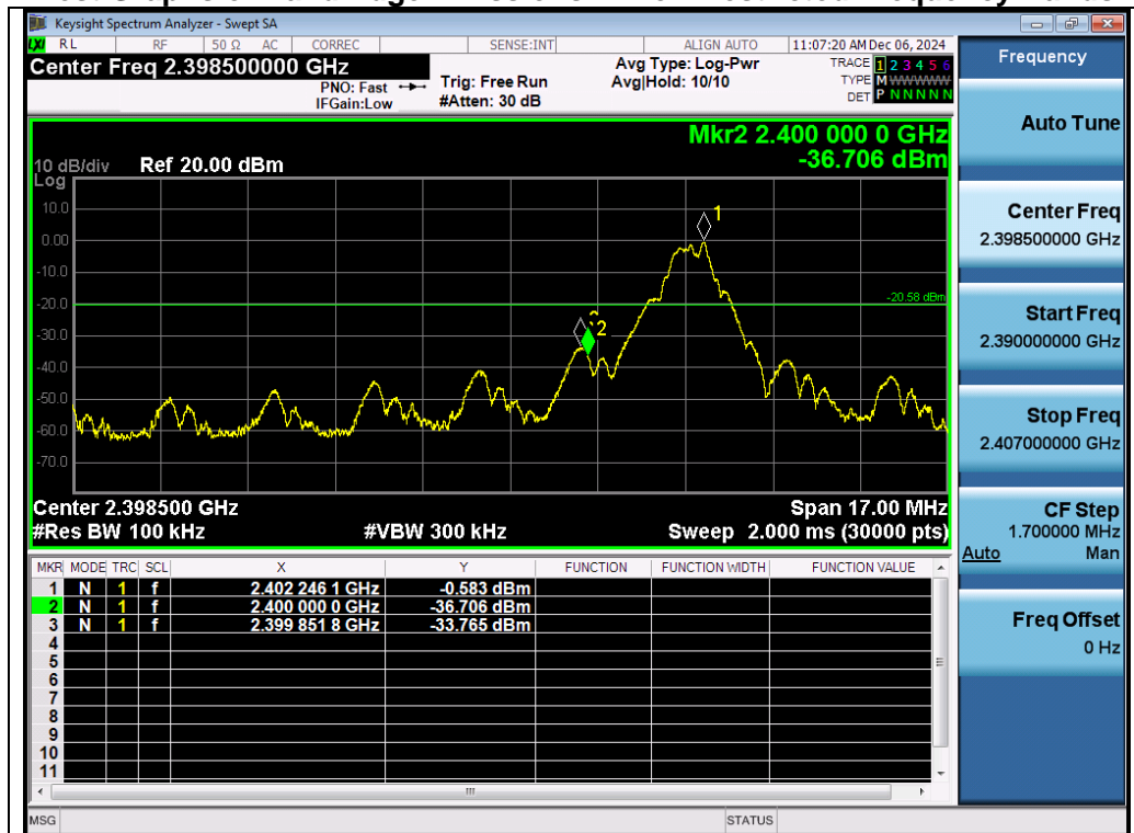
Test_Graph_LE1M_ANT1_2402_1Mbps_Lower Band Edge Emissions
