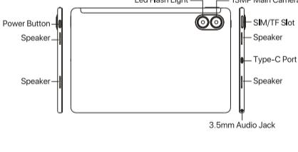
POWER BUTTON: Long press to turn on the device; When the device is on, short press Power Button to shutdown or turn on the screen.
