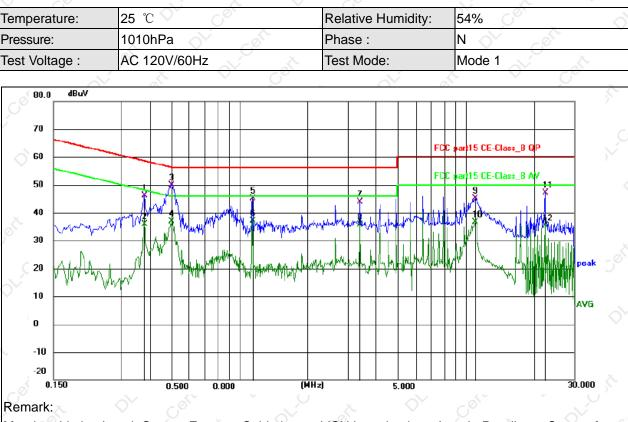
Margin = Limit – Level, Correct Factor = Cable lose + LISN insertion loss, Level= Reading + Correct factor
