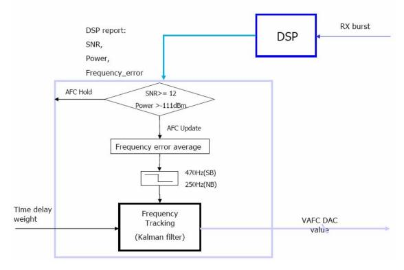
In MT6572A , it uses an AFC signal from baseband (DAC) to finish control.
