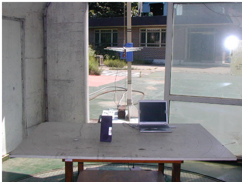
RADIATED EMISSION SETUP PHOTOGRAPH - FRONT VIEW ( 300- 1000 MHz )
