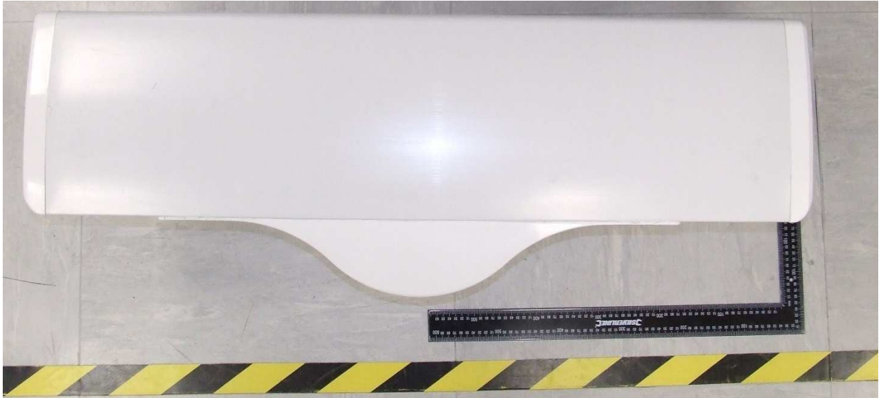
Figure 5 – Pedestal and 3ft antenna (top)
