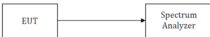
Test Setup Block Diagram
