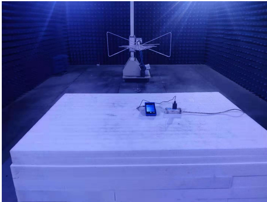
Photo of Radiated Emission Measurement (Above 1G)
