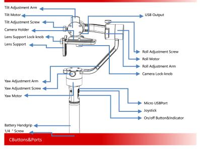
On/Off button: Single Press: Start/Stop recording Double Press: Undefined
