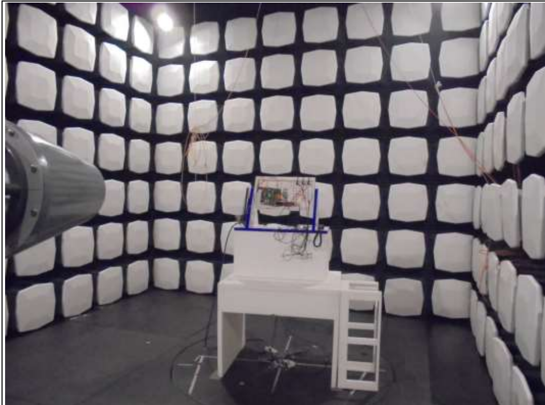
Photograph 5: Test set-up for radiated measurements (overview)
