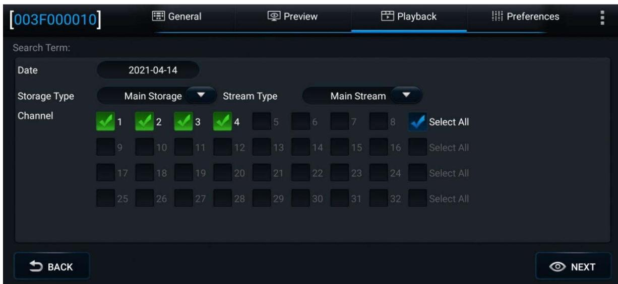
After the channel is selected, you can drag the timeline to select the playback time, and tap **Play**. During the playback, you can select the play operation. Double-tap on the screen to hide the operation screen and zoom in on the play screen.
