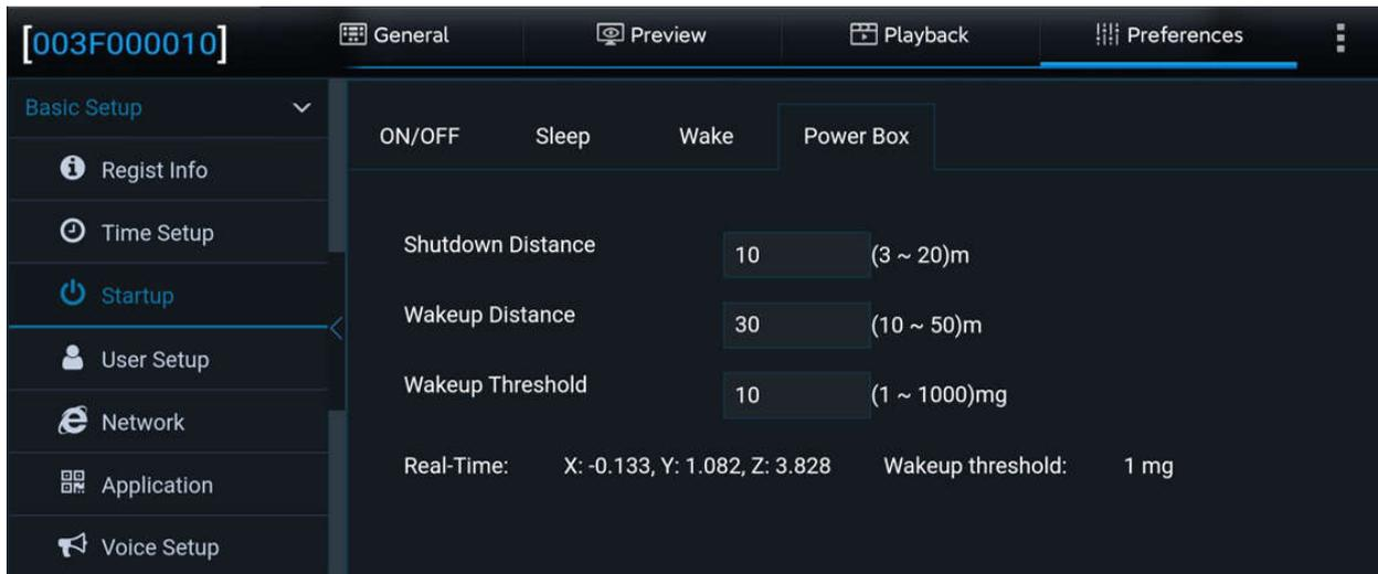
Set the shutdown and wake-up thresholds controlled by the power box
