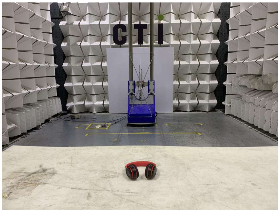
Radiated spurious emission Test Setup-1(Below 1GHz)
