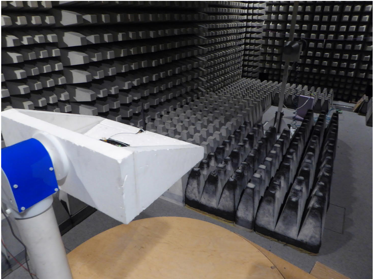
Test setup fully anechoic chamber 1 – 12 GHz
