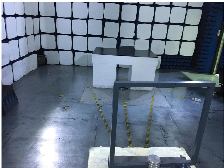
Radiation Emission Test Setup (Below 30MHz)
