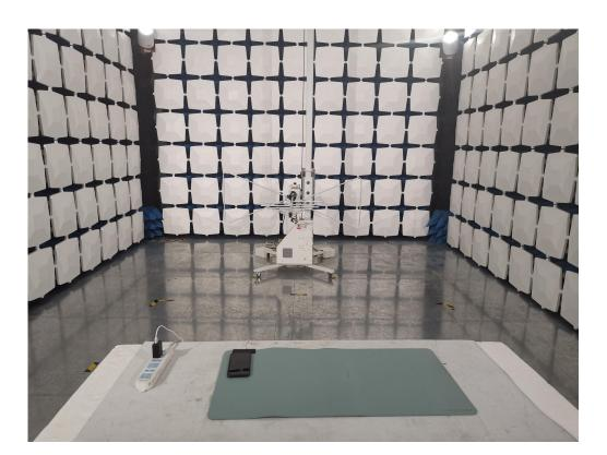
Blow 1GHz for radiated emission test setup
