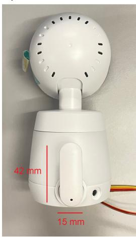
Figure 1 Physical dimension (mm)
