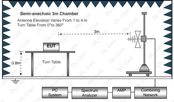
(C) Radiated Emission Test-Up Frequency Above 1GHz
