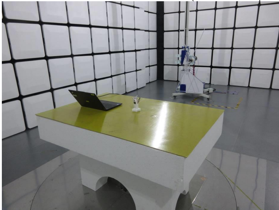
RADIATED RF MEASUREMENT SETUP (30MHz ~ 1 GHz)
