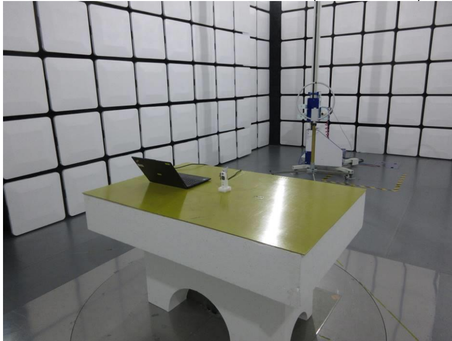
RADIATED RF MEASUREMENT SETUP (9kHz ~ 30 MHz)
