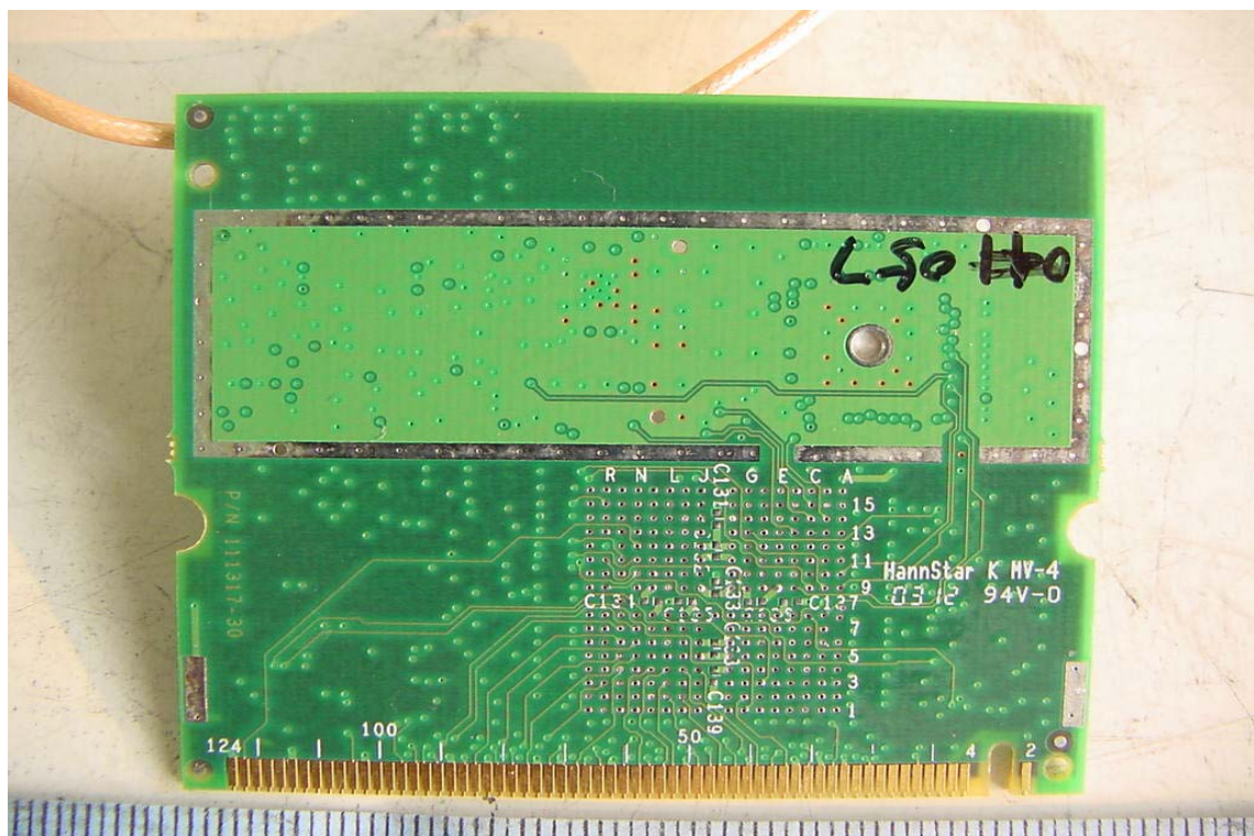
Solder View of PCB
