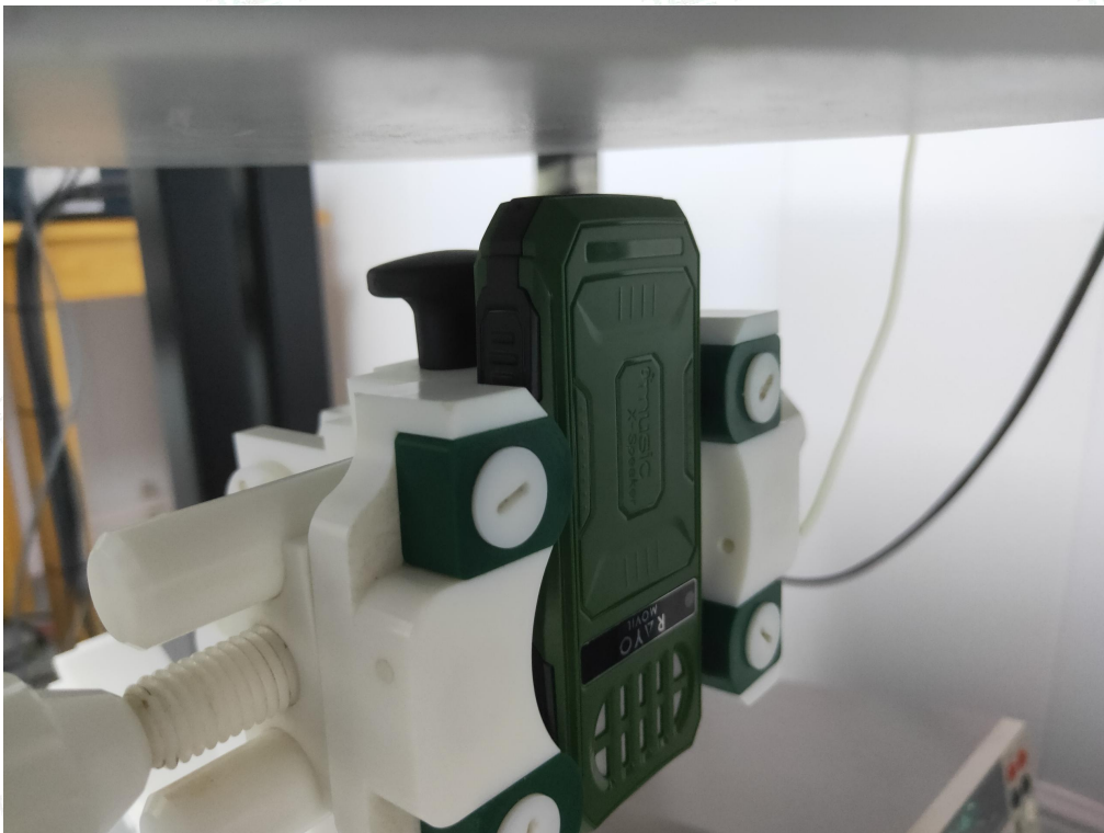
10mm body-worn Bottom Side Setup Photo (hotspot)
