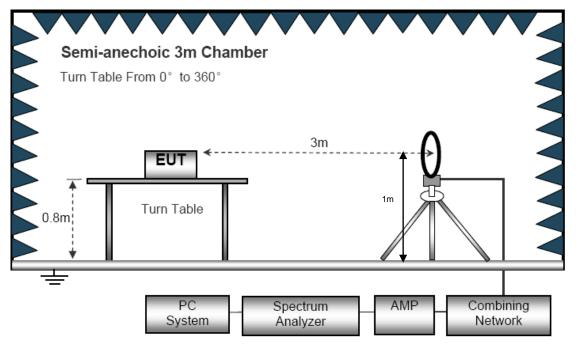
(B) Radiated Emission Test-Up Frequency 30MHz~1GHz
