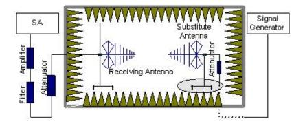
In the chamber, a substitution antenna for the frequency band of interest is placed at the reference point of the chamber. An RF Signal source for the frequency band of interest is connected to the substitution antenna with a cable that has been constructed to not interfere with the radiation pattern of the antenna. A power  $(P_{\text{Mea}})$  is applied to the input of the substitution antenna and adjusts the level of the signal generator output until the value of the
