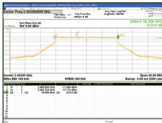
Chain0 : 6dB Bandwidth @ 802.11g Mode Ch11
