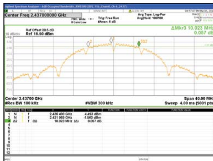
Chain0 : 6dB Bandwidth @ 802.11b Mode Ch11
