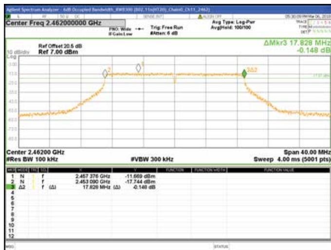
Chain0 : 6dB Bandwidth @ 802.11n(HT20) Mode Ch11
