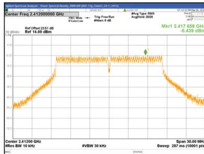
Chain1 : Power Spectral Density @ 802.11g Mode Ch 6
