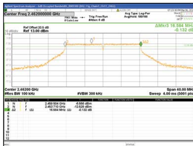
Chain1 : 6dB Bandwidth @ 802.11g Mode Ch11
