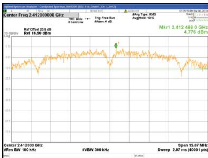
Chain1 : Conducted Spurious @ 802.11b Mode Ch 1
