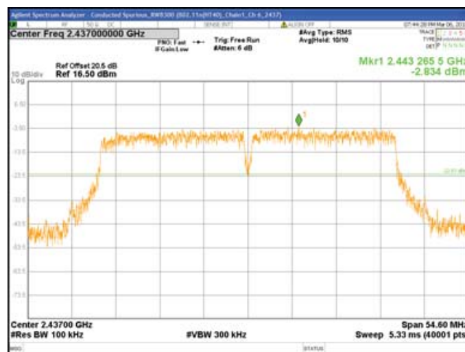
Chain1 : Conducted Spurious @ 802.11n(HT40) Mode Ch 6
