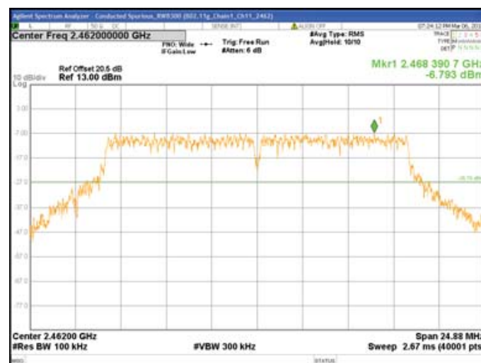
Chain1 : Conducted Spurious @ 802.11g Mode Ch11
