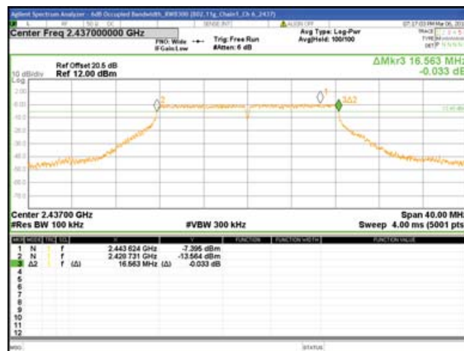
Chain1 : 6dB Bandwidth @ 802.11g Mode Ch11
