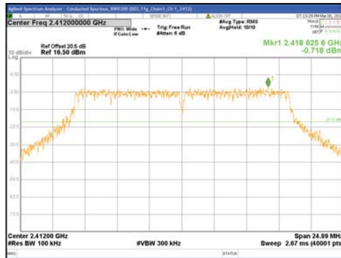
Chain1 : Conducted Spurious @ 802.11g Mode Ch 1
