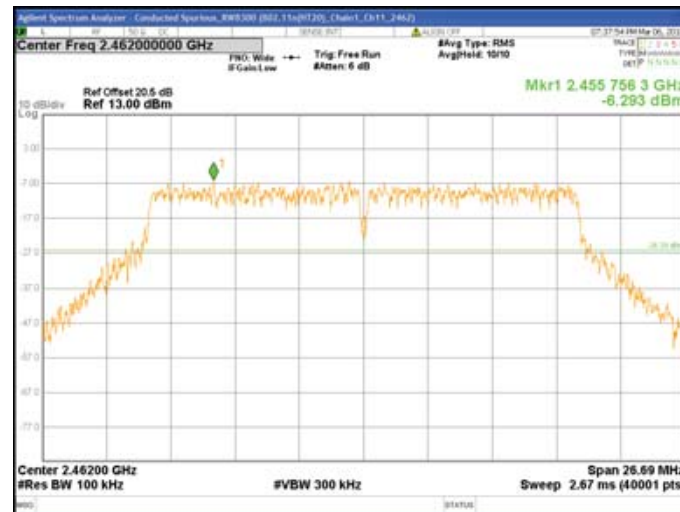
Chain1 : Conducted Spurious @ 802.11n(HT20) Mode Ch11
