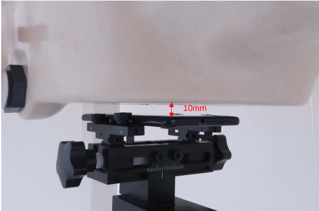
Picture 5: Back Side, the distance from handset to the bottom of the Phantom is 10mm
