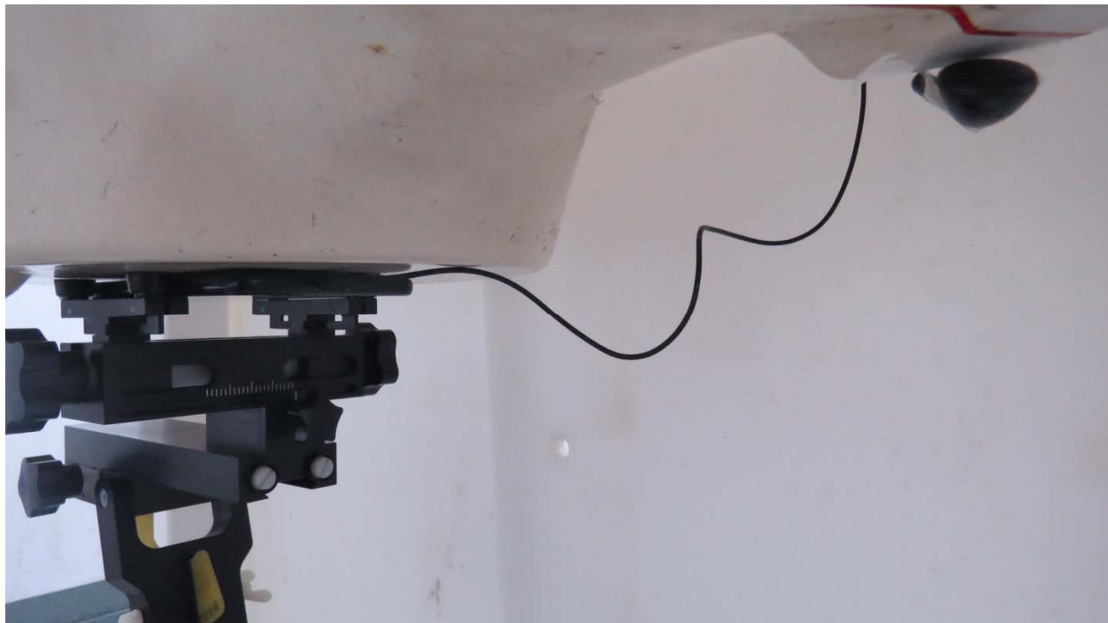
Picture 14: Back Side with Earphone, the distance from handset to the bottom of the Phantom is 0mm
