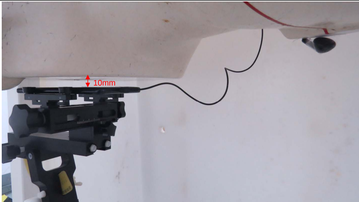
Picture 13: Back Side with Earphone, the distance from handset to the bottom of the Phantom is 10mm
