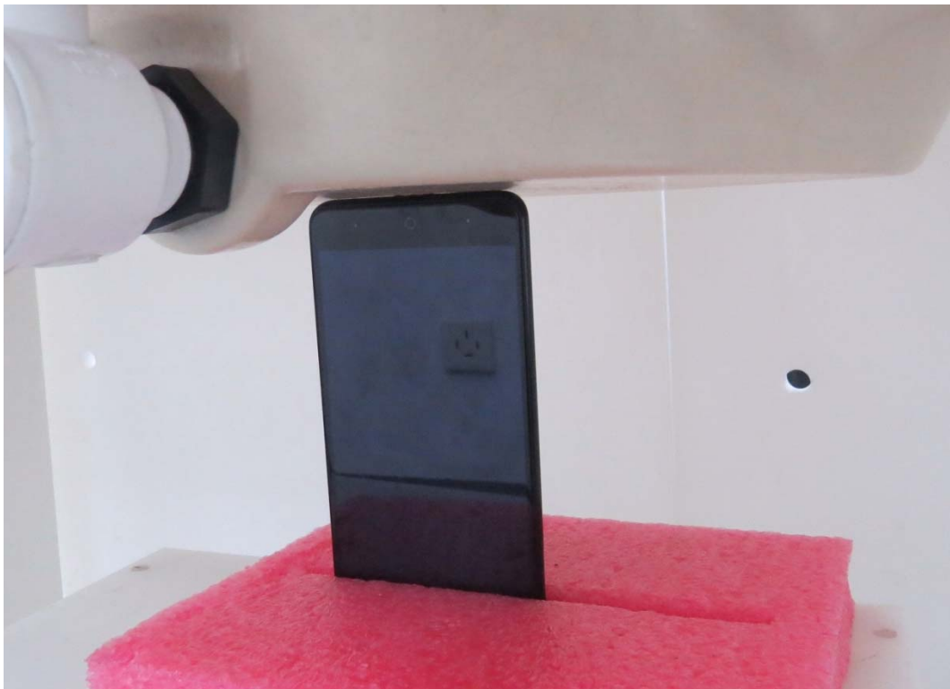
Picture 12: Bottom Edge, the distance from handset to the bottom of the Phantom is 0mm
