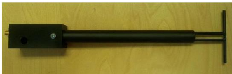
Figure 1 – MVG COMOSAR Validation Dipole
