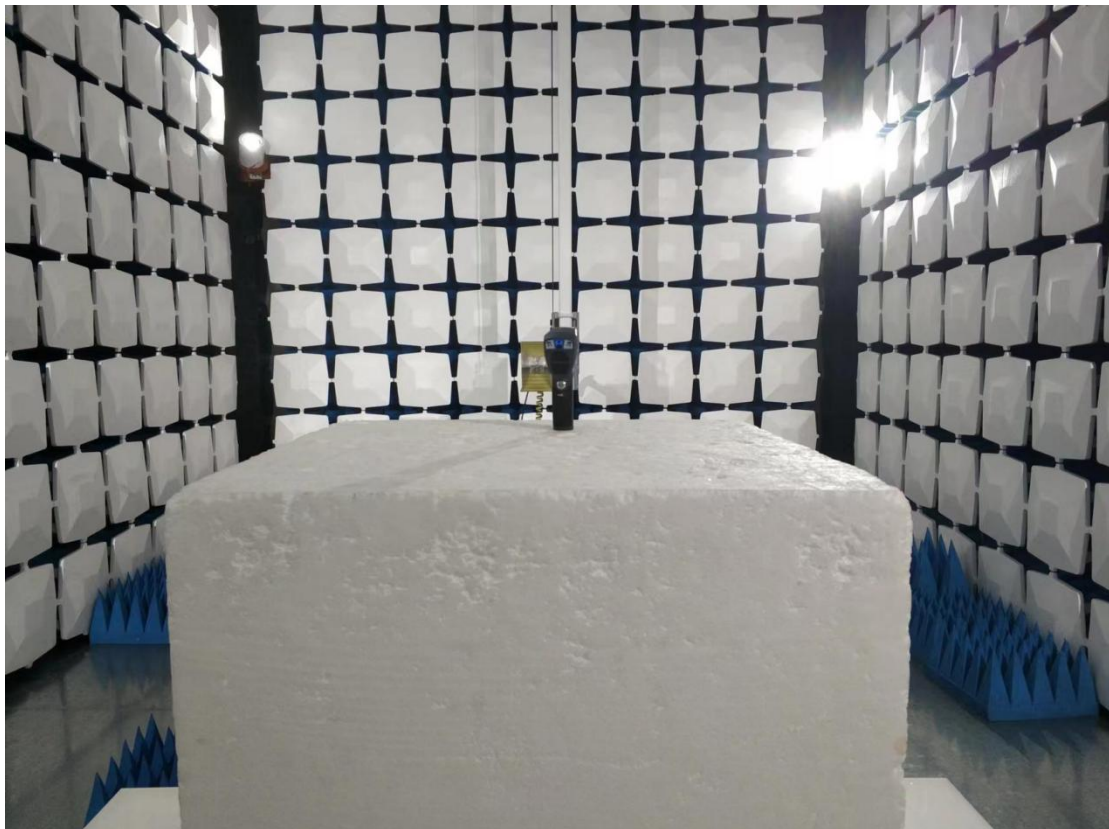
Above 1GHz for radiated emission test setup
