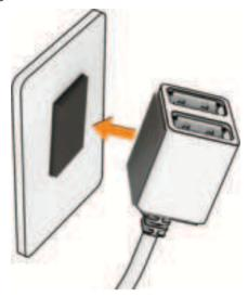
8 Connect the USB power cable from your Garmin Dash Cam device to a USB port on the Constant Power Cable device.
