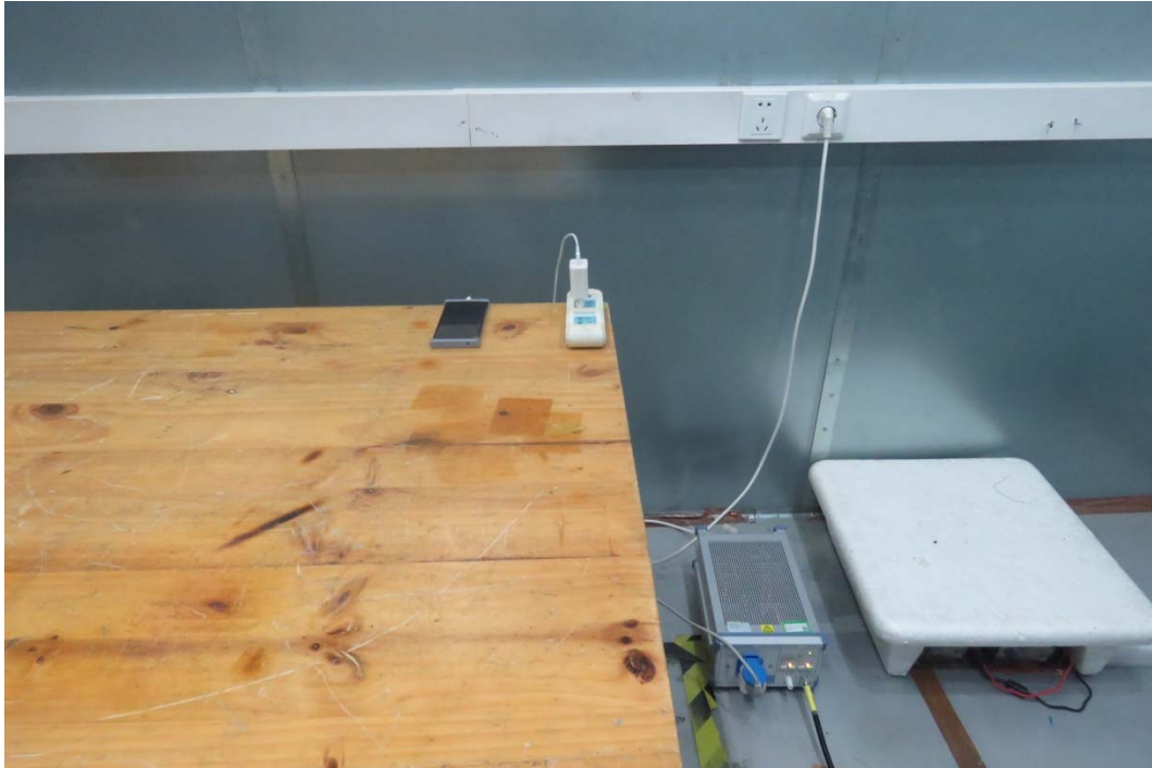
Picture 2 Conducted Emission Test Setup
