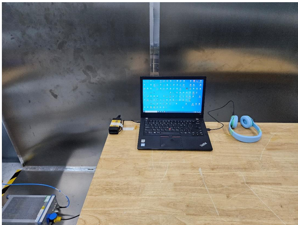
Photograph 1: Set-up for Conducted Emission on AC Mains
