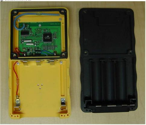
2. Top housing disassembled.
