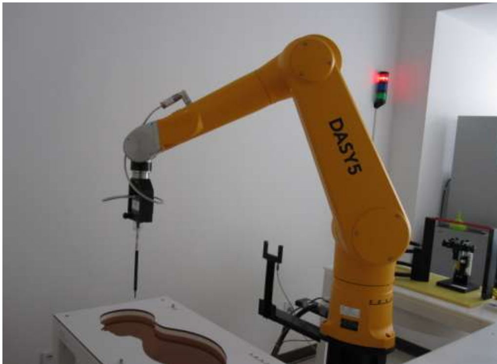
Picture C.1: Specific Absorption Rate Test Layout
