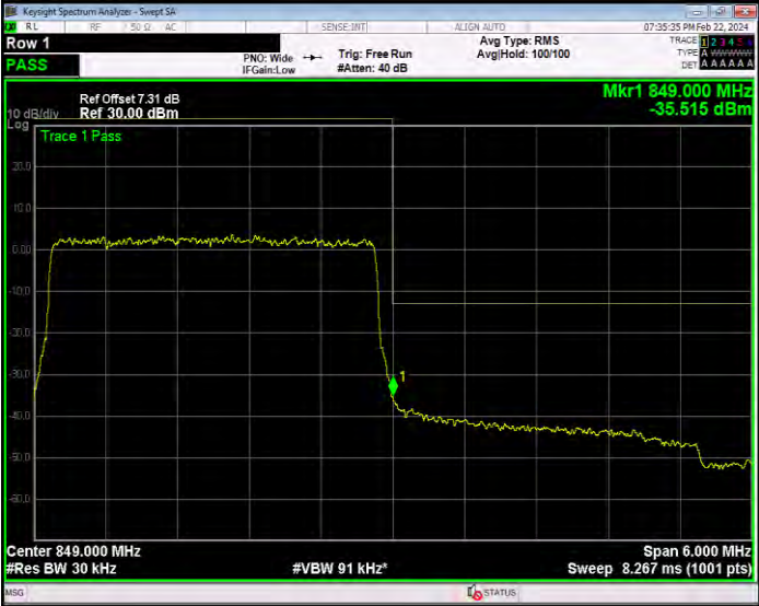
Band5 QPSK BW=5MHz Channel=20425 RB Size=1 Position=#0
