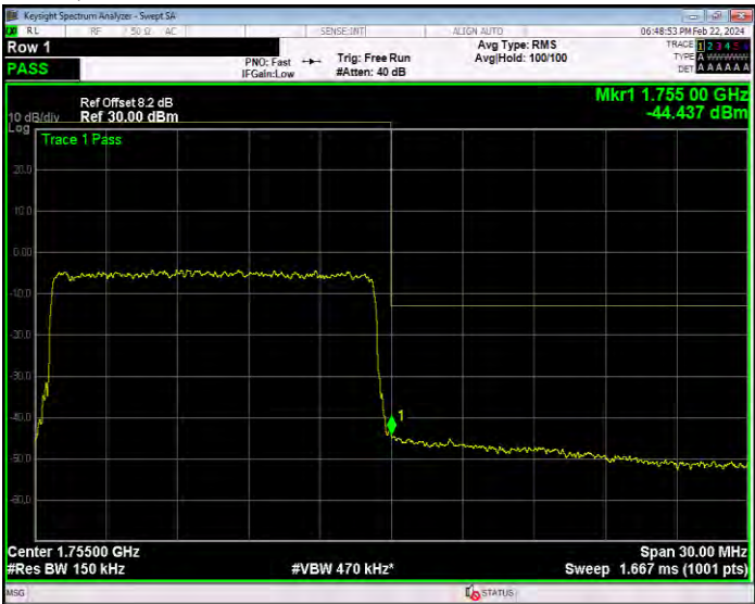
Band4 16QAM BW=15MHz Channel=20325 RB Size=75 Position=#0
