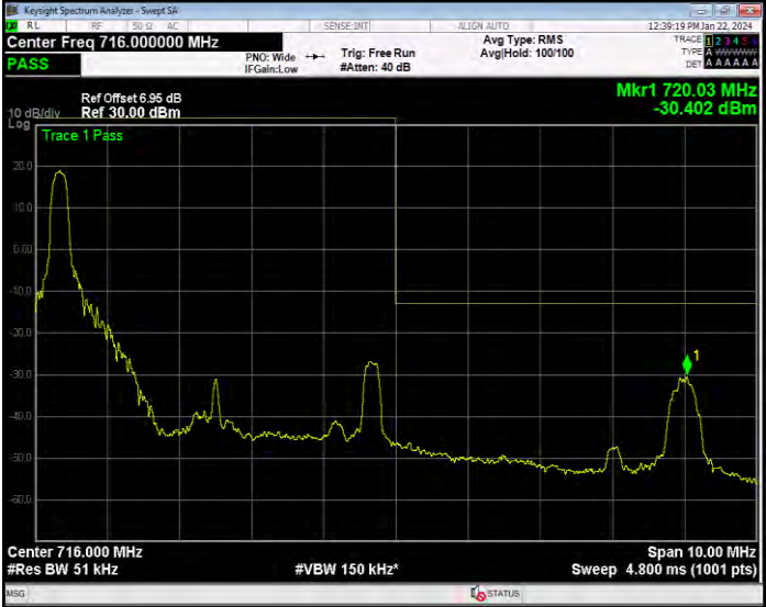
Band17 16QAM BW=5MHz Channel=23825 RB Size=25 Position=#0
