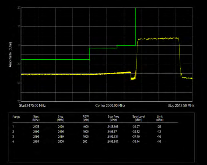
Band7 16QAM BW=10MHz Channel=21400 RB Size=1 Position=#0
