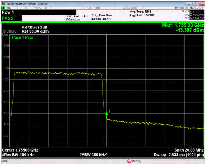
Band4 QPSK BW=15MHz Channel=20025 RB Size=1 Position=#0
