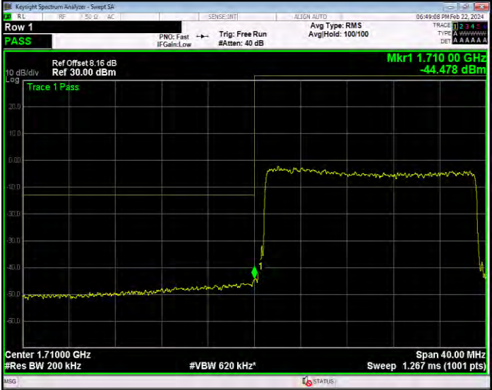
Band4 QPSK BW=20MHz Channel=20300 RB Size=1 Position=#0
