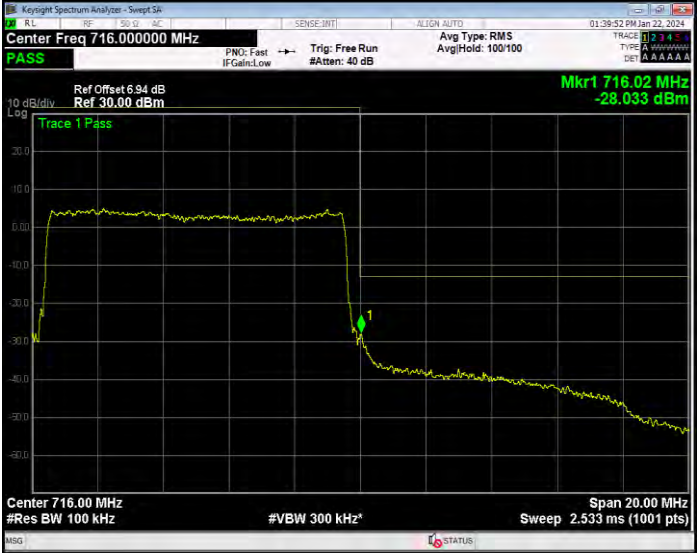
Band17 16QAM BW=5MHz Channel=23755 RB Size=1 Position=#0
