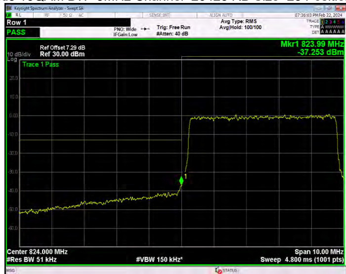
Band5 16QAM BW=5MHz Channel=20625 RB Size=1 Position=#0
