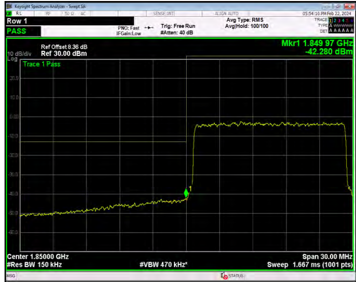
Band2 16QAM BW=15MHz Channel=19125 RB Size=1 Position=#0
