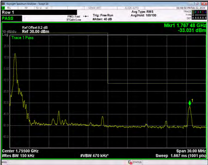
Band4 16QAM BW=15MHz Channel=20325 RB Size=75 Position=#0
