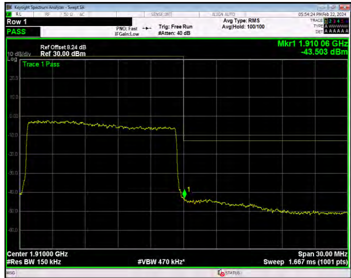
Band2 16QAM BW=15MHz Channel=19125 RB Size=75 Position=#0
