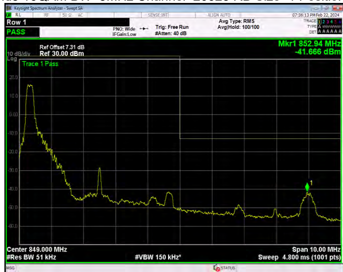
Band5 16QAM BW=5MHz Channel=20625 RB Size=1 Position=#0
