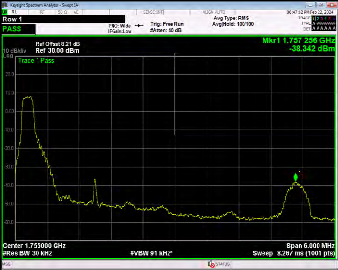
Band4 16QAM BW=3MHz Channel=20385 RB Size=15 Position=#0
