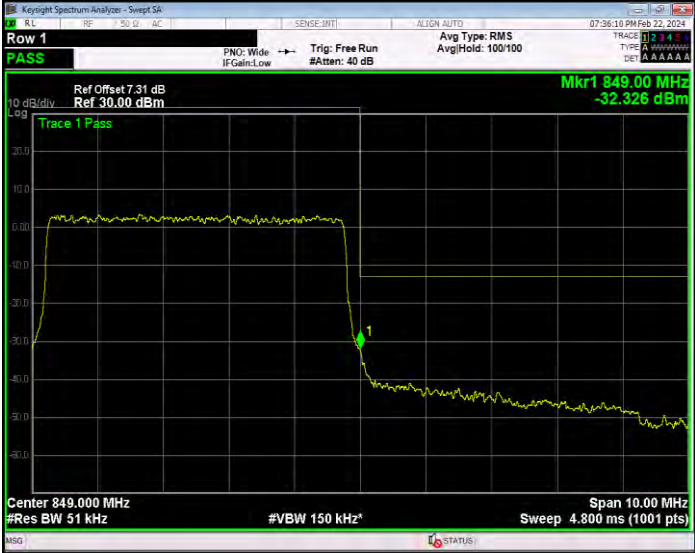
Band7 16QAM BW=10MHz Channel=20800 RB Size=1 Position=#0
