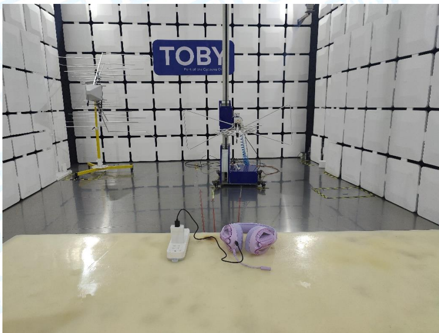
Photo of Setup for Radiated Emission (30MHz~1GHz)
