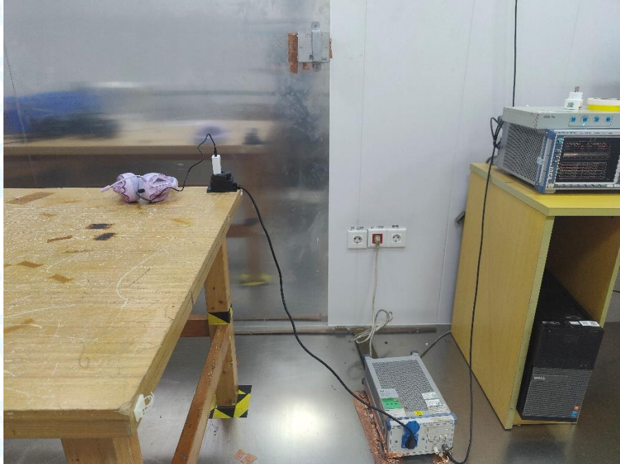
Photo of Setup for Radiated Emission (30MHz~1GHz)
