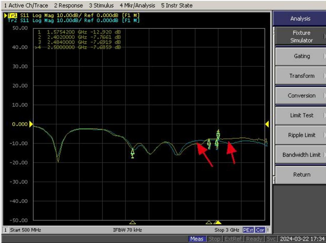
Labeling: yellow waveform if the metal ring is grounded, blue waveform if the metal ring is not grounded
