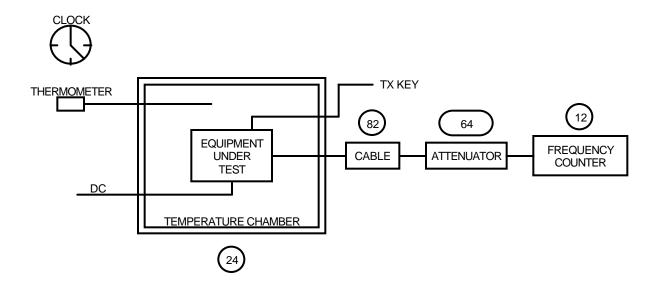
NAME OF TEST: TRANSMITTER FREQUENCY STABILITY (TEMPERATURE)
