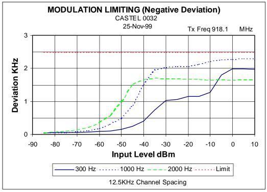
NAME OF TEST: TRANSMITTER MODULATION LIMITING
