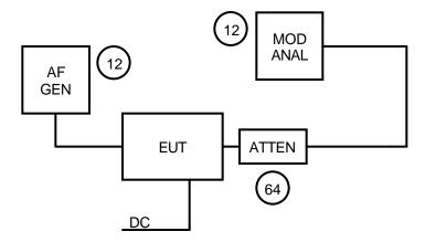
NAME OF TEST: TRANSMITTER MODULATION LIMITING
