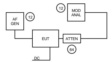
NAME OF TEST: TRANSMITTER AUDIO FREQUENCY RESPONSE
