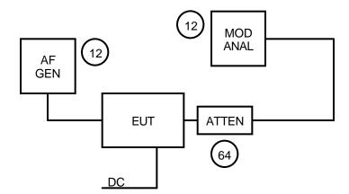
NAME OF TEST: TRANSMITTER MODULATION LIMITING
