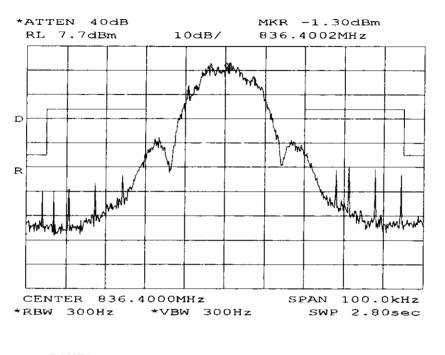
POWER: MODULATION: LOW DATA GMSK MASK: AMPS CELLULAR, F1D, DATA
