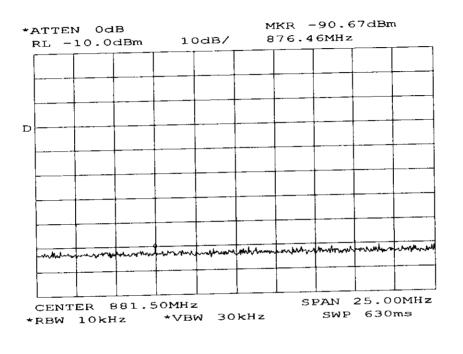
POWER: MODULATION: HIGH DATA GMSK TX SPURS IN RX CRITICAL BAND
