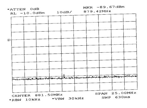
POWER: MODULATION: LOW DATA GMSK TX SPURS IN RX CRITICAL BAND
