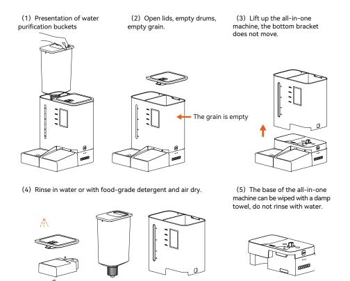
Water Tank Capacity: 4L Food Tank Capacity: 5L Power supply: DC 5V/1A Power adapter: 3 alkaline 1 batteries (batteries need to be purchased)Power supply adapted to AC110-240V input, DC5V output Product weight: 2.88kg Packing size: 31.7\*19.5\*43.5cm
