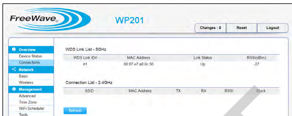
Figure 178: Connections window - WDS Bridge
