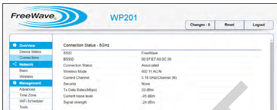
Figure 179: Connections window - WDS Station
